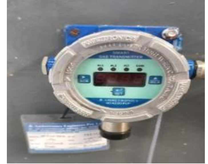
Gas Detecting Device
